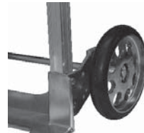
D12 8" x 1 5/8" Rubber on Aluminum Offset Hub 600 lb. Capacity (Use Short Axle)
